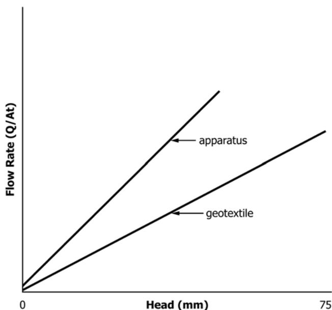
FIG. 3 Calibration Curve
